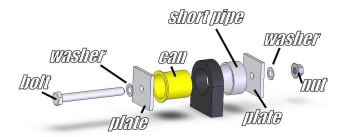
Use a  $\frac{3}{4}$ " wrench to hold the nut and a  $\frac{3}{4}$ " socket to tighten the bolt. The bolt may eventually run out of thread. When this occurs, you can replace the short pipe with the deep pipe.
