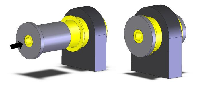
13. Install the thrust washer onto the unflanged side of the can.
