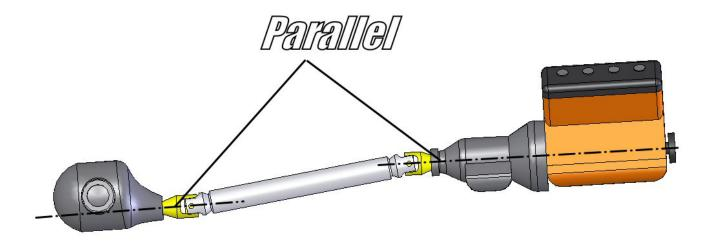
So, the first thing to do is to find out the angle the engine's crankshaft is sitting at. One way to do this is to set a digital angle finder on the front crank pulley or harmonic balancer. Record this angle. Next, set the digital angle finder on the front flat face of the differential yoke. This angle needs to be the same as the recorded crank angle. Adjust your Hotchkis trailing arms to obtain the angle needed.
