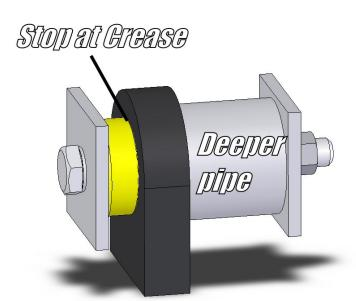
Press the metal can in until it reaches the crease.
