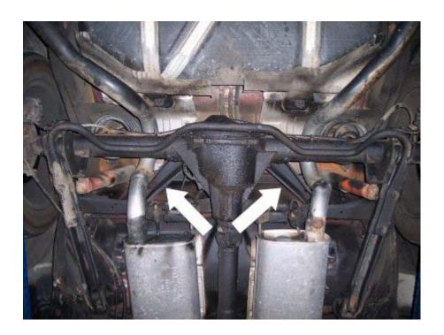
8. Now here comes the difficult part; removing the stock Can Bushings. These are the bushings that connect the aft end of the upper trailing arms to the differential. You may luck out and be able to hammer them out with a dead blow hammer, but if you are not able to use this method please do the following.
