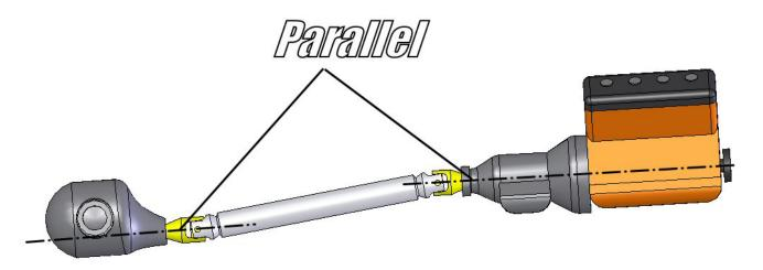
FYI... The centerlines should not be the same line because the U-joints would wear in the same areas all the time. Having an angle at the joint itself allows the joint to articulate and wear evenly along the entire bearing race.
