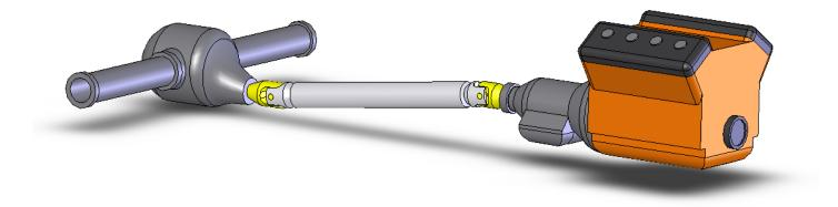
The Hotchkis double adjustable trailing arms allow you to adjust the pinion angle with ease. Simply loosen the two jam nuts and rotate the aluminum turnbuckle to lengthen or shorten the arm. So, how does one set the pinion angle?
