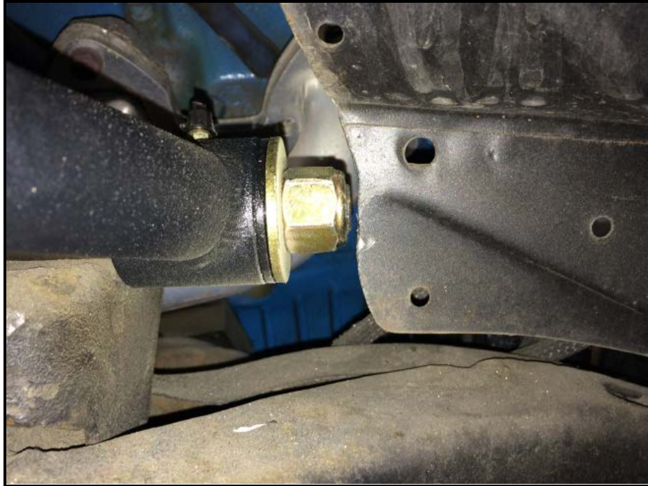
Tighten Cross Shaft bolts Completely
