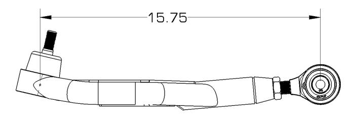
Start with the inner mounting point. You will need to insert the provided stainless steel spacer between the clevis mount and the Hotchkis swivel joint. Tighten this bolt down.
