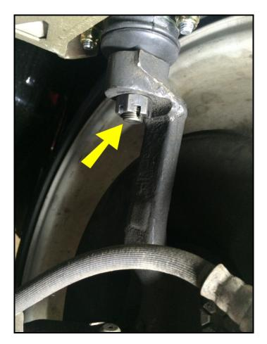
The ball joint stud is taper pressed in the spindle mount. To remove the stud from the spindle force and/or impact is required to break the press fit. There are a number of ways to do this, but the best method is to make an inexpensive tool with off the shelf components. Go to the hardware store and pick up two 3/4" x 1.75"long
