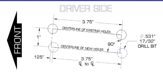
Basically the new bolt pattern is 1" down and 1/8" towards the rear of the car. These dimensions are orthogonal to the centerline of the existing holes.
