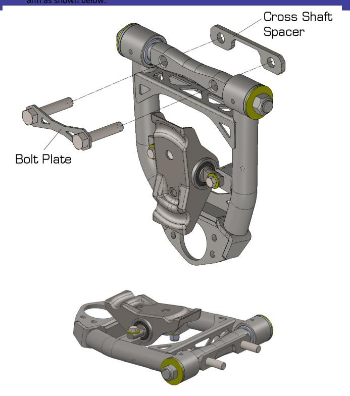
Install the arm onto the vehicle. Do not worry about using alignment shims at this point. You will need to align the vehicle after the installation is complete anyways. Fasten the bolt plate using the provided washers and nylock nuts. Repeat the steps 1-7 in reverse order to complete the install.
