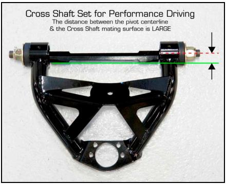
There are two possible orientations for the cross shaft. The top picture shows the position for normal street driving conditions, where below -1.5° of camber is desired. The lower picture shows the cross shaft flipped to gain an additional -1.5° of camber for performance alignments. Each car may vary.
