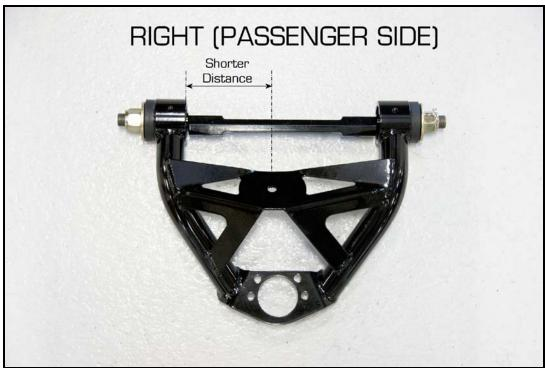
Pictures above show how to determine which side is which. The droop stop hole and the bushing tube can be your reference point.
