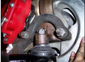
**18. Reinstall the Steering Tie Rod**Reinstall the steering tie rod in the same manner as removal. Don't forget to install the cotter pin.
